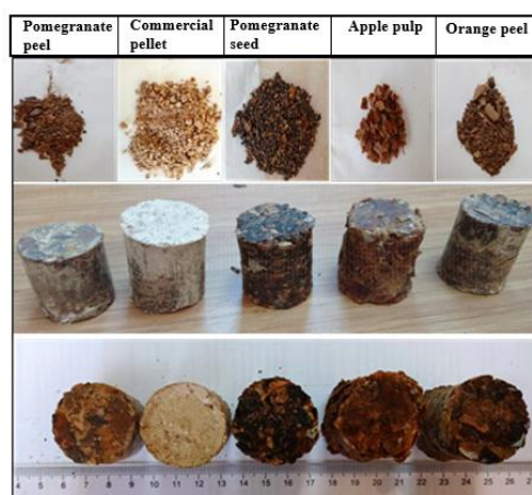
Figure 3. Experimental pellet samples
