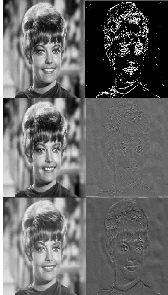
Fig 5 Wavelet decomposition (level 2). Top: input image (left) and decision map (right). Middle: approximation (left), horizontal detail (right) images in adaptive mode. Bottom: approximation (left), horizontal detail (right) images in non-adaptive mode
