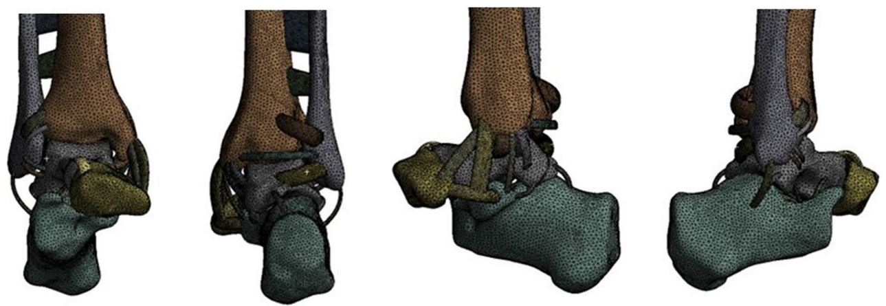
Fig. 4 Mesh structure model; the reference model contained 677,386 tetrahedral elements and 1,082,100 nodes
