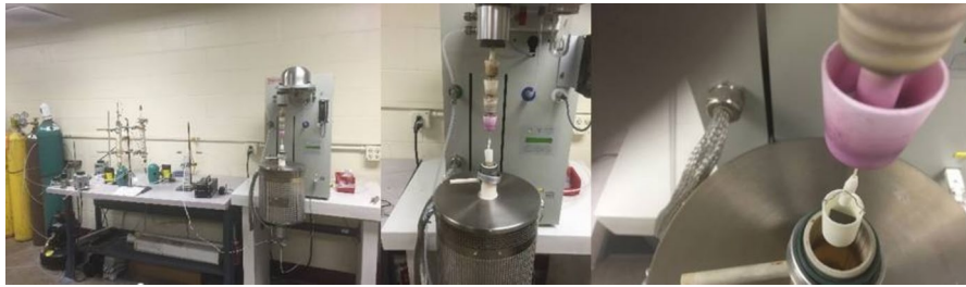
Fig. 2 Photos of the experimental system for oxidation studies using TGA
