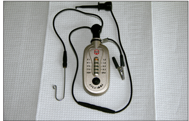
Figure 3. Electronic apex locator Apex D.S.P. (Septodont, France)
