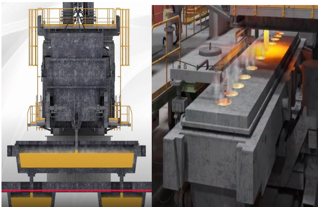
Figure 3. Slab Casting flow ladle to tundish
